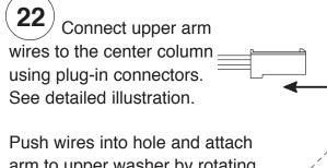
arm to upper washer by rotating arm into place. Lock down by tighting screws into flange.
