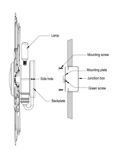
2. Fasten the ground wire to the green or bare copper wire in the junction box or the green screw on the mounting ring.
