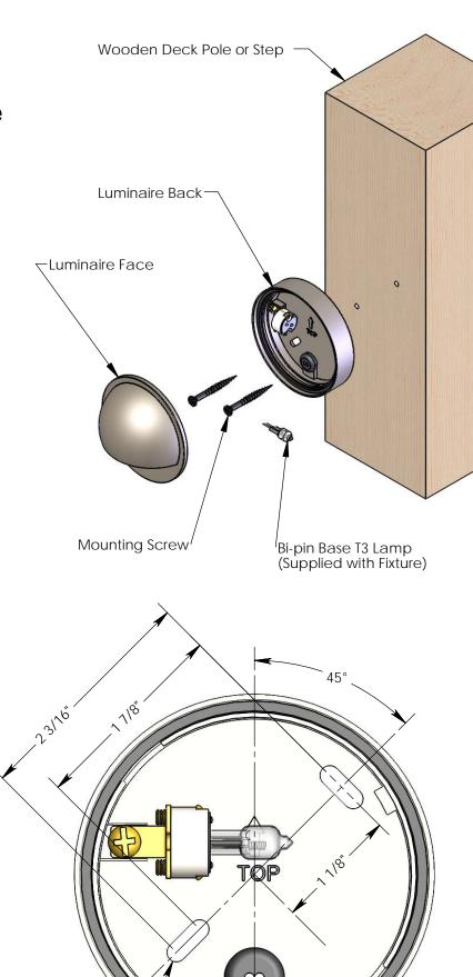
Drilling Template Full Scale
