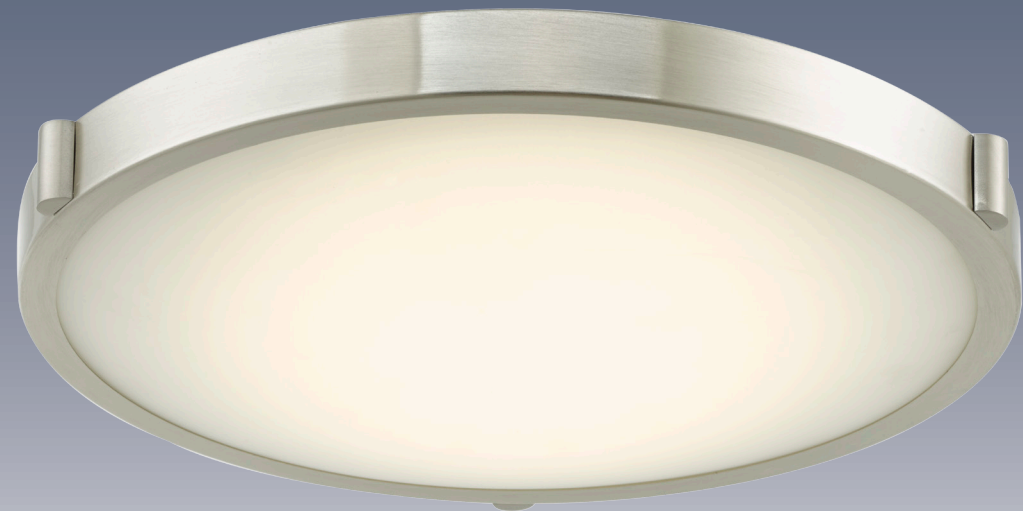
30067FM-BN | 1 x 29w LED 3000k 90+ CRI | Total Wattage 29w | 2320 Initial Lm | 2000 Delivered Lm | D 16.8" H 2.8"
