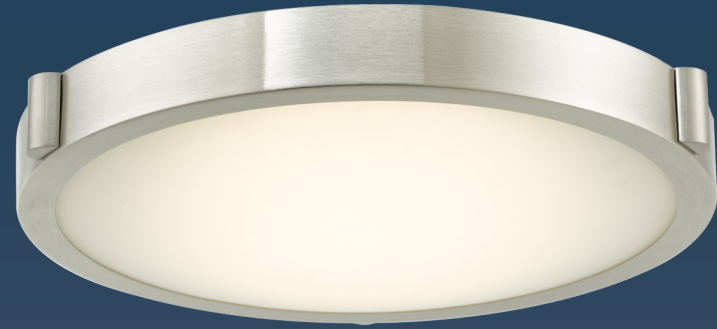
30065FM-CH | 1 x 16w LED 3000k 90+ CRI | Total Wattage 16w | 1280 Initial Lm | 1100 Delivered Lm | D 10.8" H 2.8"
