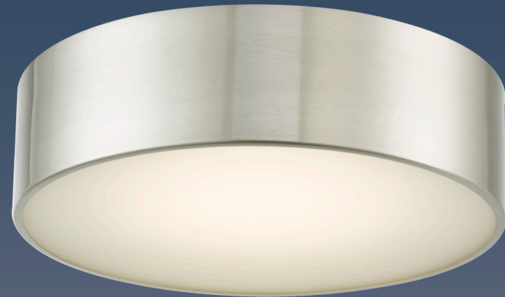
30031FM-BN | 1 x 20w LED 3000k 90+ CRI | Total Wattage 20w | 1600 Initial Lm | 1380 Delivered Lm | D 12.0" H 3.4"
