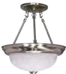
11" Semi-Flush Convertible to Pendant (2) 60W A19 max. / Medium Base Dimensions: Width 11 3/8", Height 12", Wire 12' 60-200 Brushed Nickel / Alabaster Glass Accessories: 25-1403 Pendant conversion kit 25-1069 3' Section of matching chain
