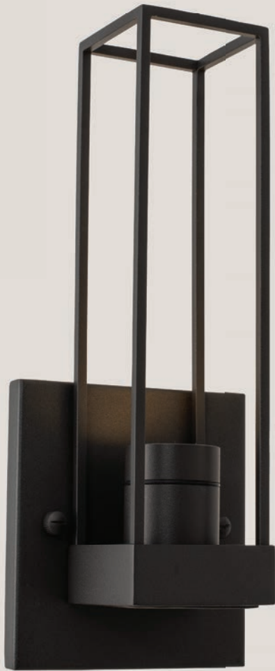
405021 MB SHORT ADA LED WALL SCONCE W: 5 H: 11 E: 4 5.5W / 3000K / 800 LUMENS
